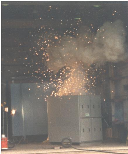
Figure 3. Successful arc test on 15 kV metal-clad switchgear.
