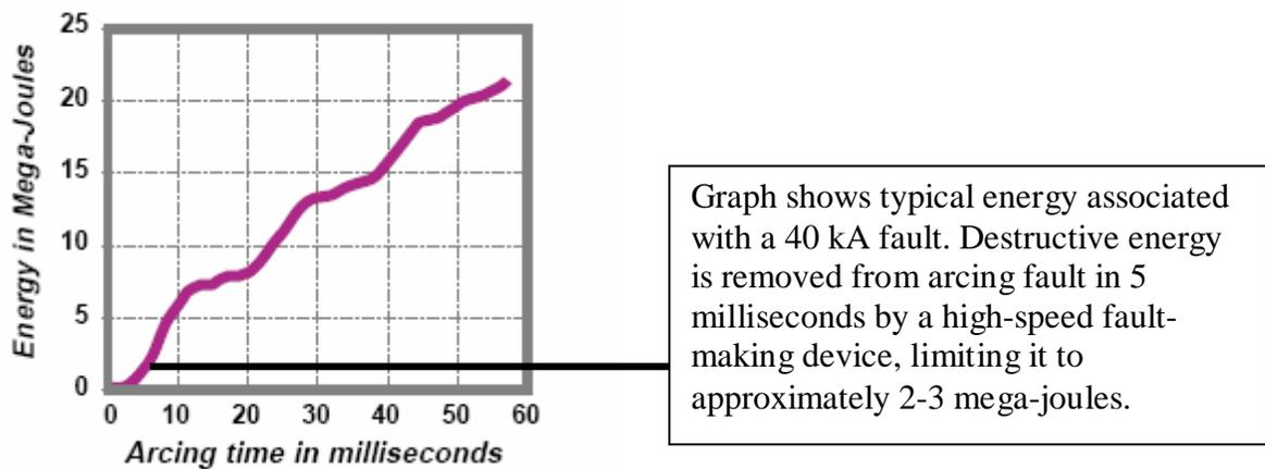
Figure 5. High-speed fault-making device limits destructive energy significantly
